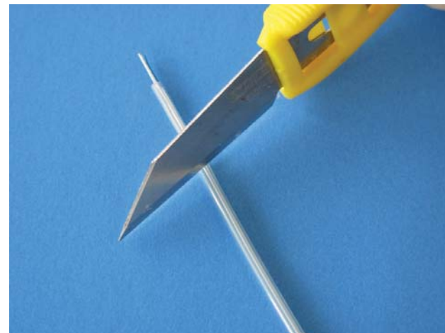
Using scalpel or other device carefully remove lead's outer insulation.
