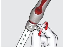
Retract the needle completely into the sheath and lock the thumbscrew on the safety ring at the 0 cm mark.
