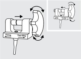
The firing position allows the handle to be rotated in the forward direction only. The **two-way position** allows the handle to rotate in both directions. Prior to introducing the endoscope, keep the handle in the two-way position.
