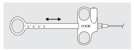
Fully retract and extend the snare to confirm smooth operation.
