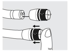
Attach the barrel to the tip of the endoscope, advance as far as possible.
