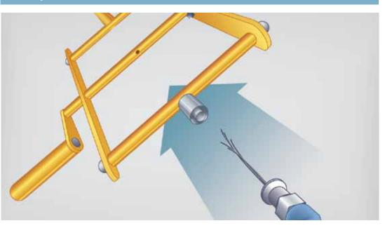
Pass the basket wires through the male Luer lock on the lithotripsy handle; and through the rotating rod opening of the handle.
