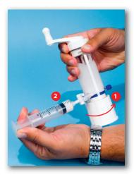
Rotate base of mixer to close the port by raising the o-ring
