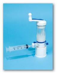
Attach a 20 cc syringe with a standard 3-way stopcock to uncapped port
